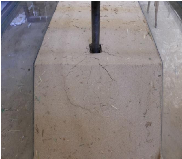
Fig. 4 Slope Failure (Slope 1H: 1V, R.S = 0.5% and X = 6 cm)
