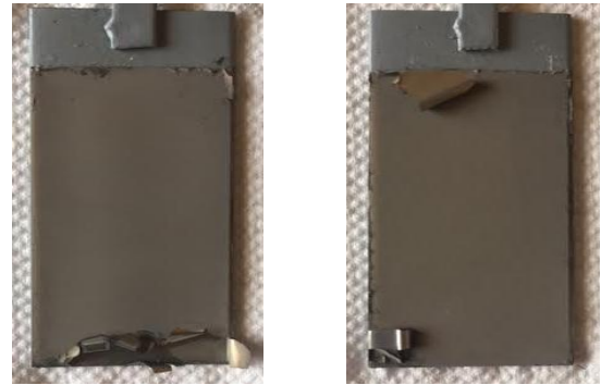
Figure (1): The Damage in surface layer by electrodeposition using times above 6 minutes at (40 mA/cm 2 )
