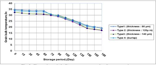
Fig. 3. Change in grain bulk temperature as related to storage time.
