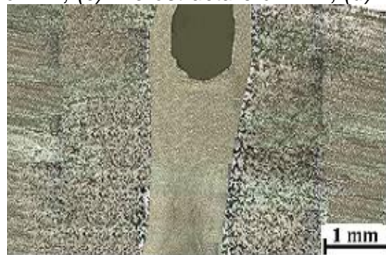
Figure (4). Optical micrographs showing fusion boundary of the worst sample
