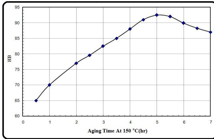
Fig. 3 Hardness as a function of aging time during one-stage aging at 150 °C
