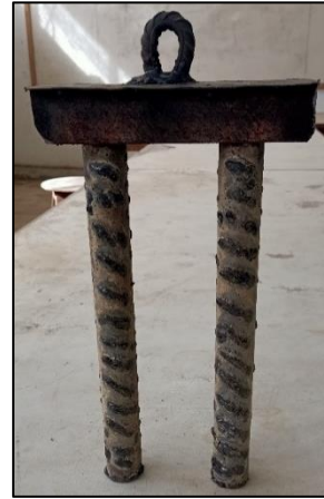
Fig. 3. The model of the pile group with a spacing of three times the single pile diameter used in the present study.
