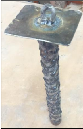
Fig. 2. The model of the circular steel pile with bulges used in the present study.
