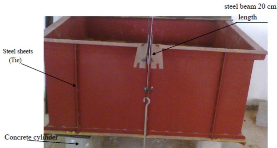
Fig. 1. The metal box (mold) for soil sample preparation.
