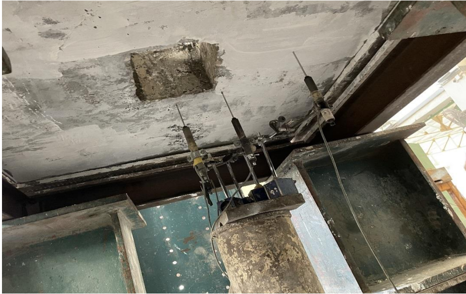
Fig. 7. Adjusting the dial gauges at bottom surface of specimen for measuring deflection (LVDT).
