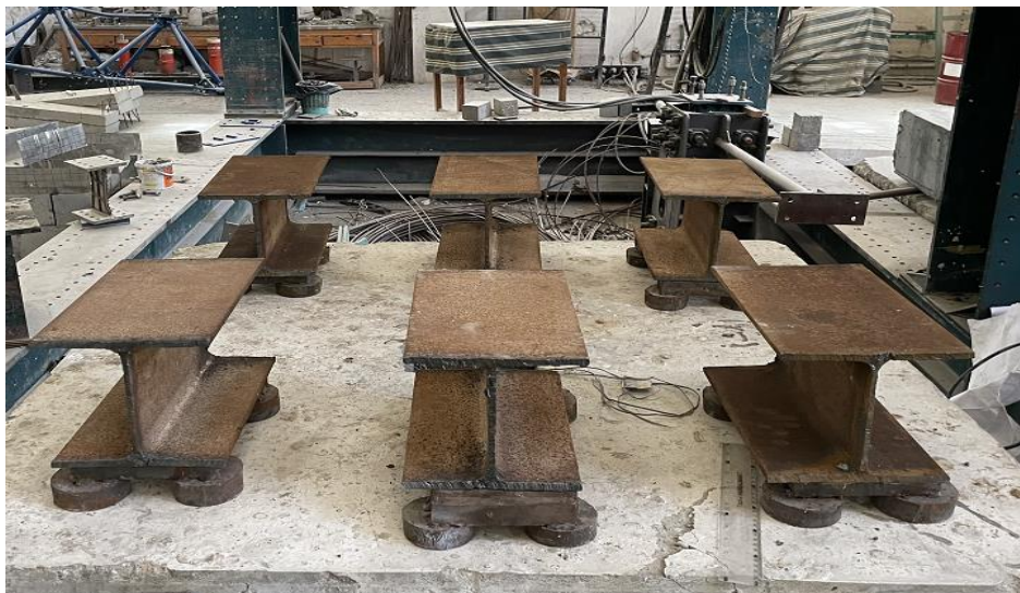
Fig. 6. Uniform load distribution point.
