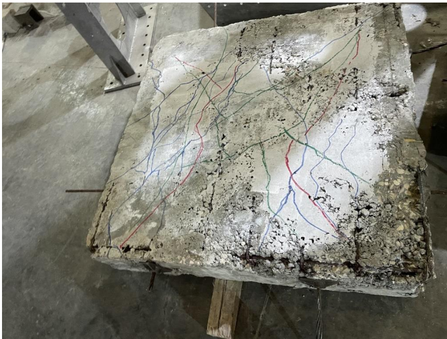
Figure. 14. Crack behavior of slab (S6).
