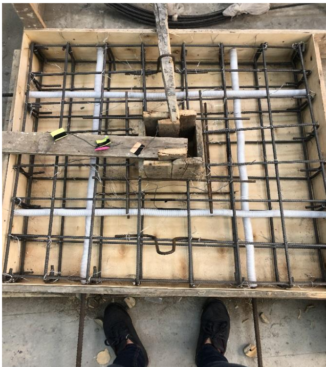
Fig. 4. Typical Steel arrangement details of PT slab S6 and strands distribution, with opening 25*25 cm.
