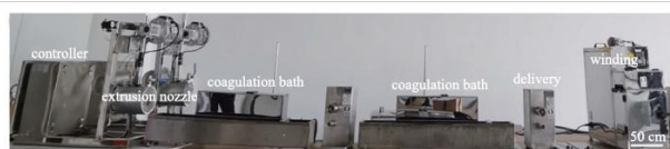
Figure 7: A continuous spinning mechanism used to create thermochromic fibres [54]
