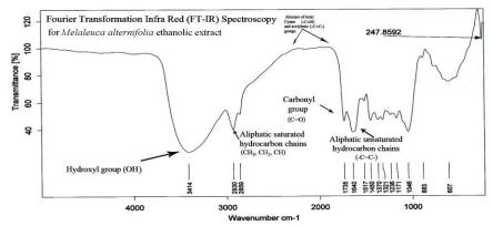
Fig. 4. FT-IR profile analysis for Melaleuca alternifolia methanolic leaf extract.
