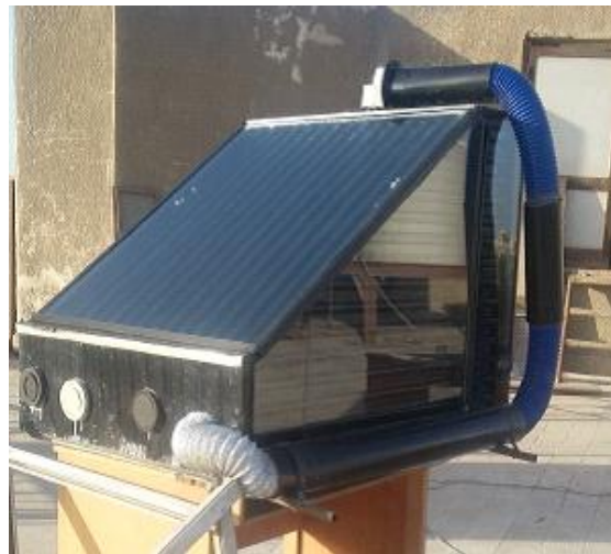
Figure 2. The developed solar dryer with three sides flat plate solar collector.
