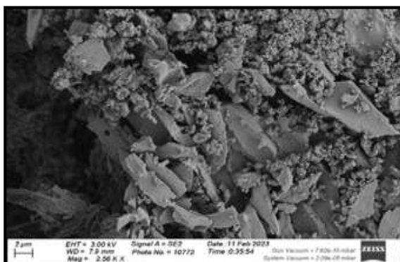
Figure 1. Scanning Electron Microscopy (SEM) of BCs derived from sugarcane bagasse at 300 and 600 °C (BCBG 300 vs. BCBG 600 ) and sugarcane filter- cake at 300 and 600 °C (BCFC 300 vs. BCFC 600 ) at 300 and 600 °C, respectively.
