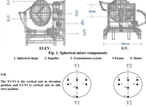
Fig. 2. Location of ash measuring points
