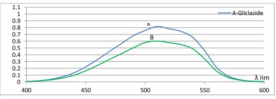
Fig. (2) Absorption Spectra of methyl Orange in presence of 12µg/ml Gliclazide (A) and 8µg/ml Glibeneclamide (B).
