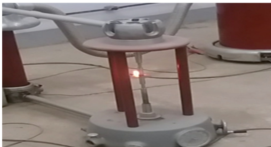
Fig. 1 . Specimen under effect of flashover voltage test.
