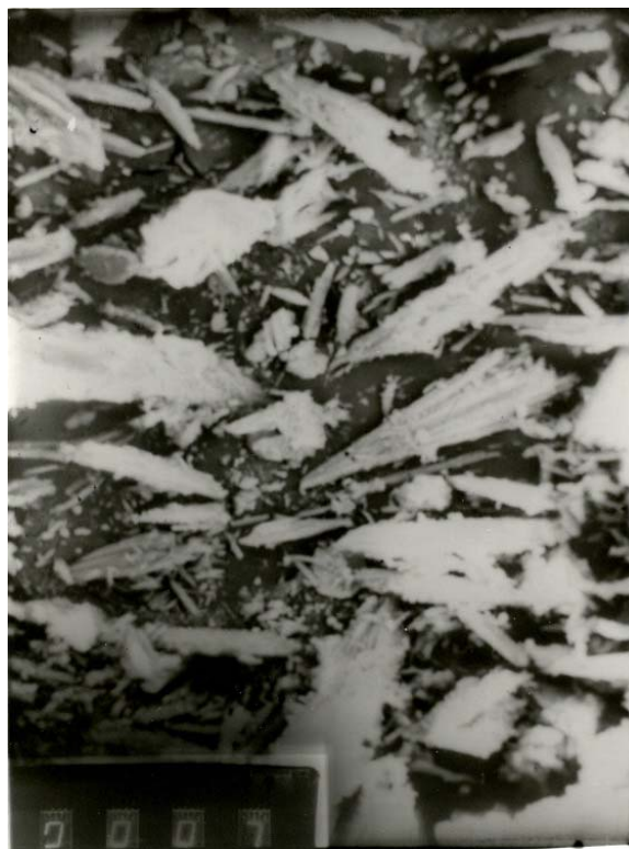
Fig. 4: SEM micrograph of PACSi-SO 4 X100
