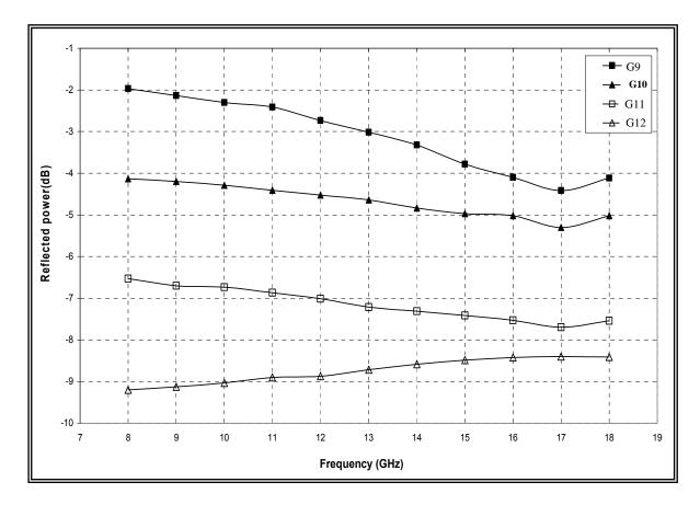
Fig.4. Relation between the frequency and reflected power of cotton-polyester (40%-60%) textile fabric with different concentration of graphite in shellac solution
