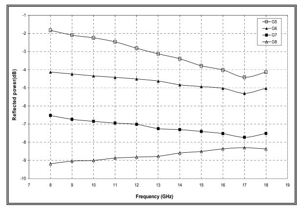
Fig.3. Relation between the frequency and reflected power of 100%cotton textile fabric with different concentration of graphite in epoxy polymer.
