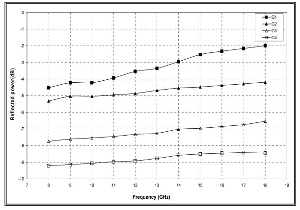
Fig.2. Relation between the frequency and reflected power of 100%cotton textile fabric with different concentration of graphite in alcoholic shellac solution.
