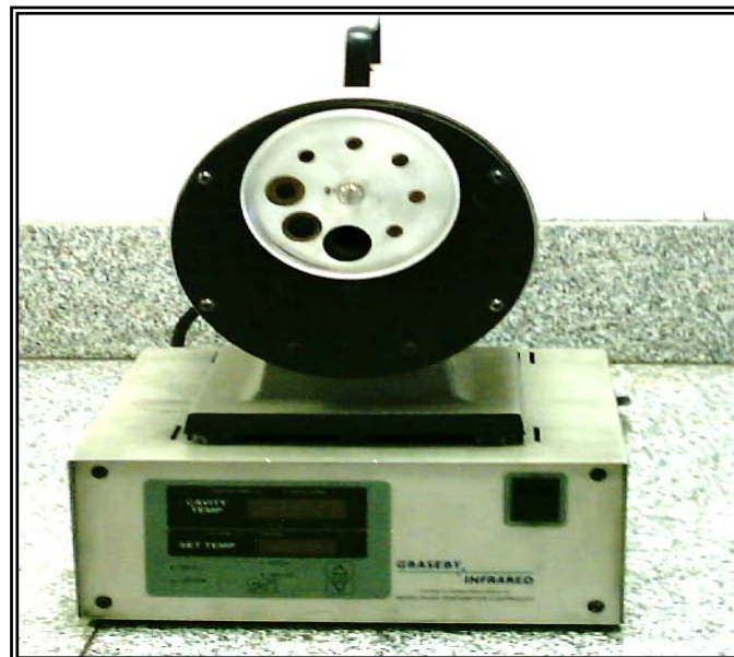
Figure (2.4) Graseby infrared black body radiator with temperature controlling unit
