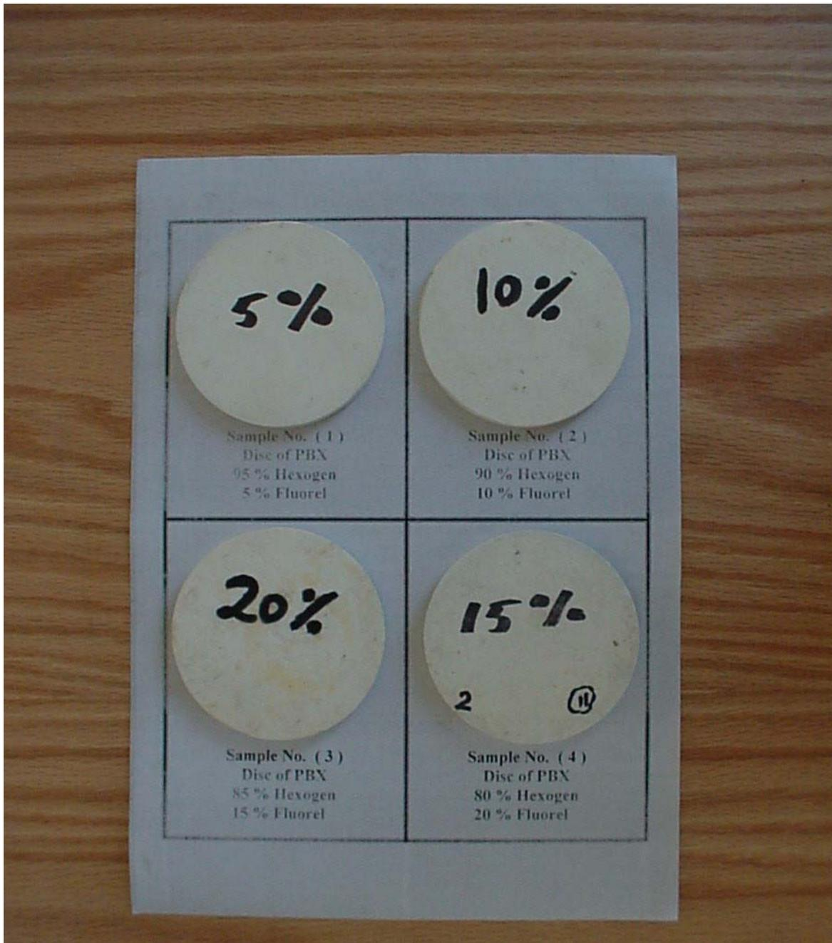
Fig. 1. Photograph of the prepared PBXs Sheets
