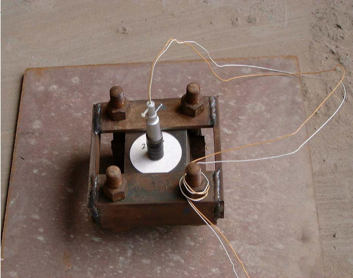
Fig. 4. The set-up of the jet attack test
