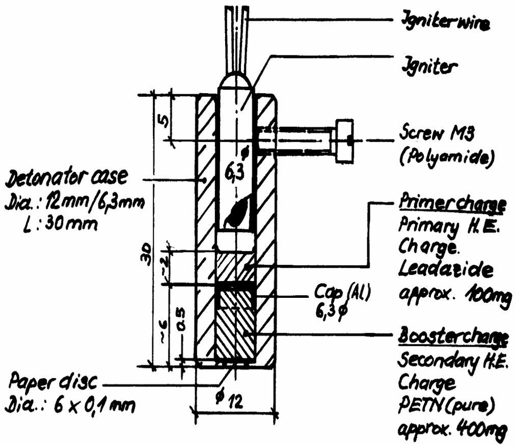
Fig. 2. Cross Section of the used detonator
