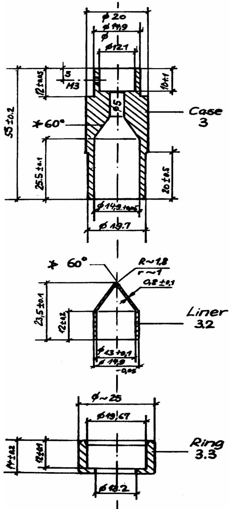
Fig. 3. Main components of the used shaped charges
