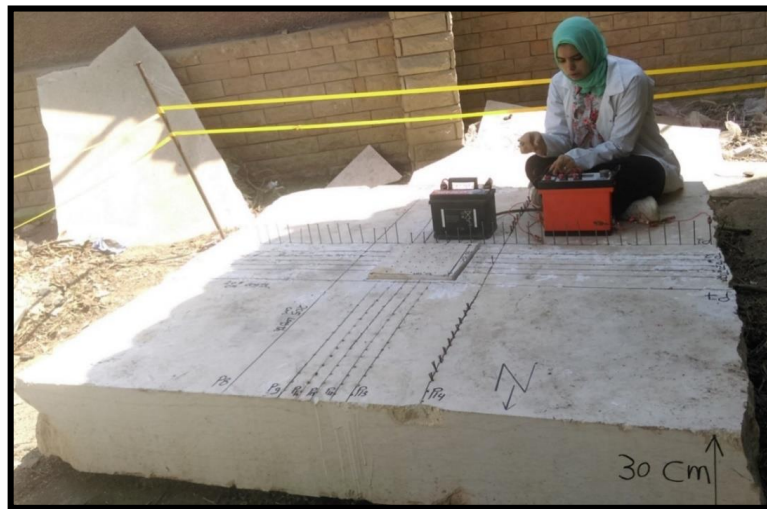
Fig. (2): Resistivity data acquisition during the laboratory measurements on the top of the limestone model, 10 cm long metal electrodes were used for both sounding and profiling.
