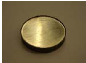
Fig. 2. As-hot compacted sample
