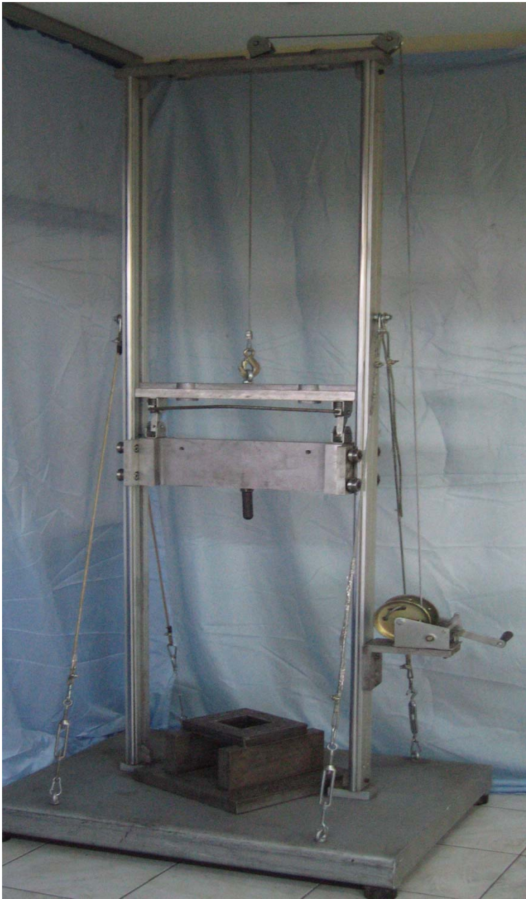
Fig. 1. Instrumented falling weight impact test machine.
