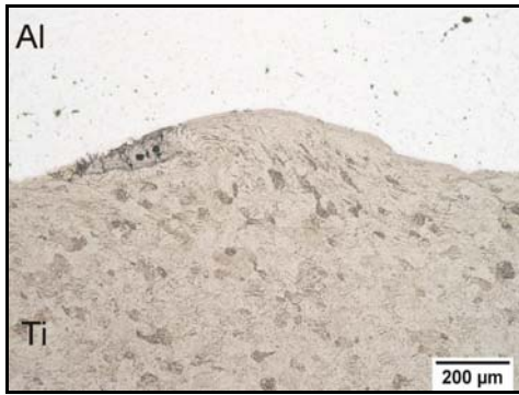
Fig. 13. Microstructure of Ti – Al interface (Keller etching).
