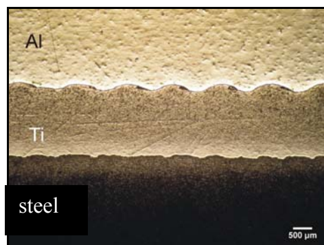
Fig. 12. Macrostructure of trimetal (section perpendicularly to the Ti – steel explosion direction and in the Al - Ti explosion direction).
