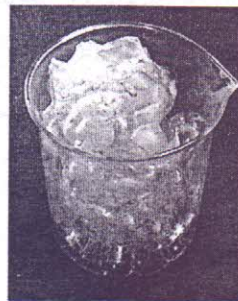
Fig.1 Etching the limestone slice by HCl 5%
