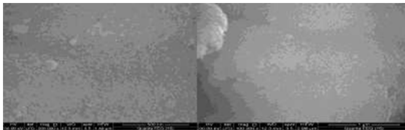
Fig. (4). Scanning electron microscope of iron nano-composite with \text{TiO}_2 .
