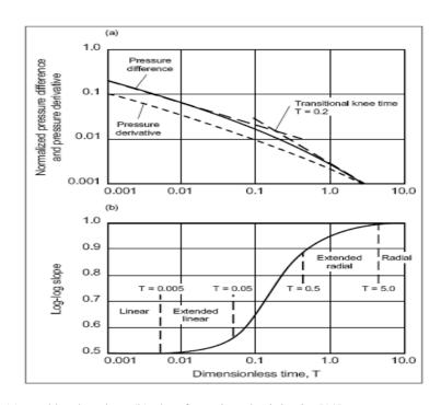
(a) and log-log slope (b) plots for an impulse injection[11] Figure 2 After-Closure pressure difference and derivative
