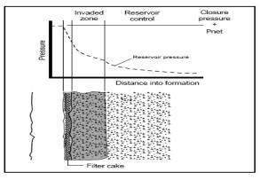
**Figure 3** The three regions of fluid loss between fracture and reservoir[11].
