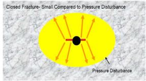
Figure 5 Flow pattern of Radial flow period for after closure [12].
