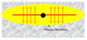
**Figure 4** Flow pattern of linear flow period for after fracture closure[12].
