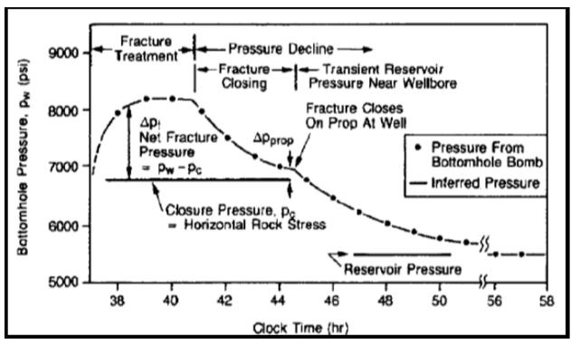
Figure 1 Typical History of Calibration test (Nolte[4][5]).
