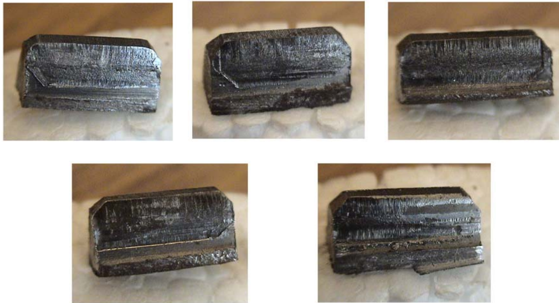
Fig. 10. View of the Tooth Samples Cut Away From the Gears Pertaining to Gear Samples of 48 Teeth, 49 Teeth, 50 Teeth, 51 Teeth and 52 Teeth. These Gears Represent Tooth numbers Alterations of Z_e = -4, -2, 0, +2 and +4 .
