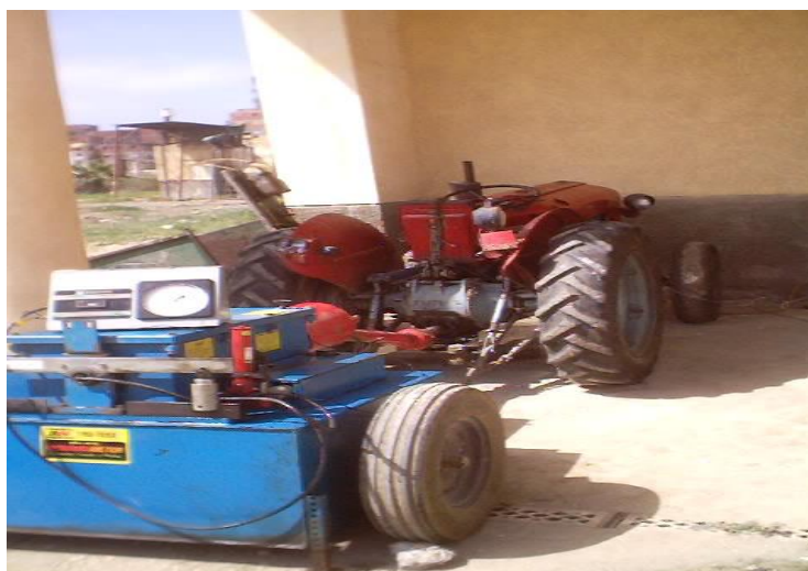
Figure 1: The tractor PTO was coupled to the dynamometer for applying loads
