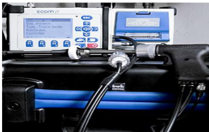
Fig. (3): The exhaust gas analyzer
