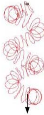
Figure 01: Twin helical spring filament subjected to axial force \vec{T}
