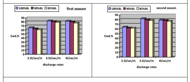
Fig.3 :Water distribution efficiency (Ewd, %) as affected by the combination of discharge rates and cut-off irrigation treatments during the two growing seasons
