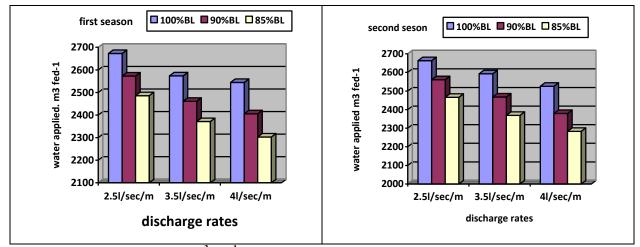
Fig. 1: Seasonal applied water (m<sup>3</sup> fed<sup>-1</sup>) for wheat crop as affected by discharge rates and cut-off irrigation treatments during the two growing seasons
