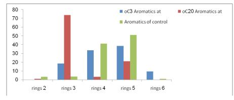
Fig. 3. Polyaromatics distribution of control crude oil and polyaromatics separated at 20°C and polyaromatics separated at 30°C.
