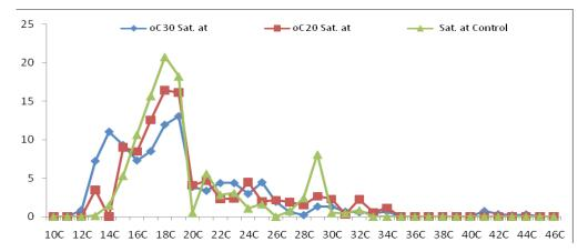
Fig. 2. Distribution of saturates for control crude oil and saturates separated at 20° C, saturates separated at 30 ° C.
