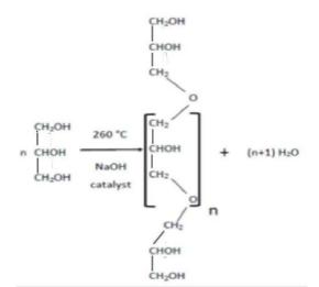
reaction with other molecules of glycerol or other polymerized molecules. The reaction produces polymers which are almost entirely linear [19]. Care must be taken during the polymerization reaction to exclude air from the system. Traces of oxygen lead to the formation of acrolein as well as a dark product which is not easily bleached.
