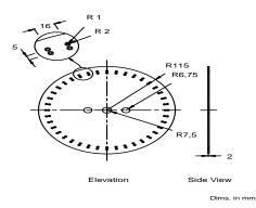
Fig. 1: Schematic diagram of the vertical grain plate.
