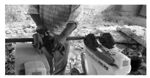
Fig. 5: A rearward curve furrow opener 3. Field Test Experimental field design
