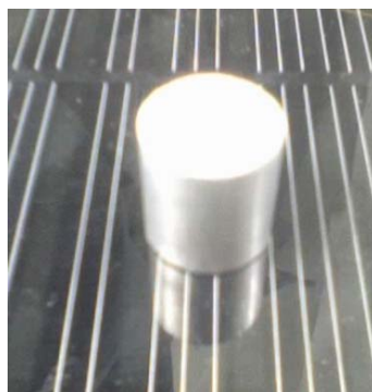
Fig. 1. Compacted A356 aluminum alloy
