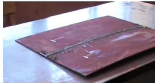
Fig. 6 : plate buckling deformation after welding and cooling (AH36) (experimental work)
