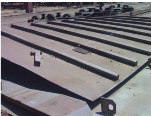
Fig. 2. The resulted warping distortion and deformations in a weldment.
