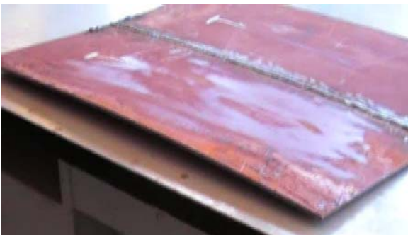
Fig. 6 : plate buckling deformation after welding and cooling (AH36) (experimental work)
