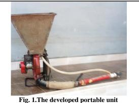
The developed portable unit consists mainly of the grain hopper, broadcasting device and power system. The specifications of each part could be discussed as follows:
