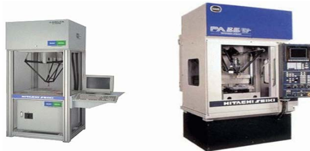
Fig.6. Hitachi Seiki's Delta robots for pick-and-place and drilling (Courtesy of Hitachi Seiki) [4]
