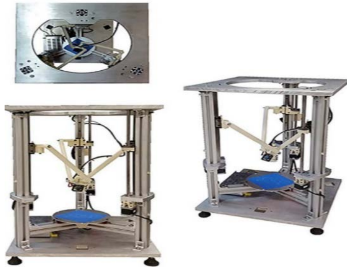
Fig.17. The fabricated aluminium prototype of the LDr-AM [26].
