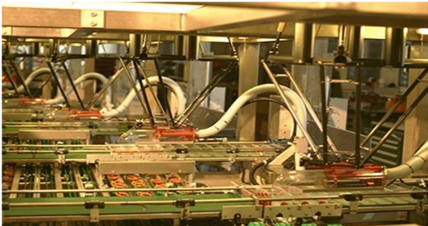
Fig.4. Demareux's Line-Placer installation for the packaging of pretzels in an industrial bakery (courtesy of Demareux) [4].
