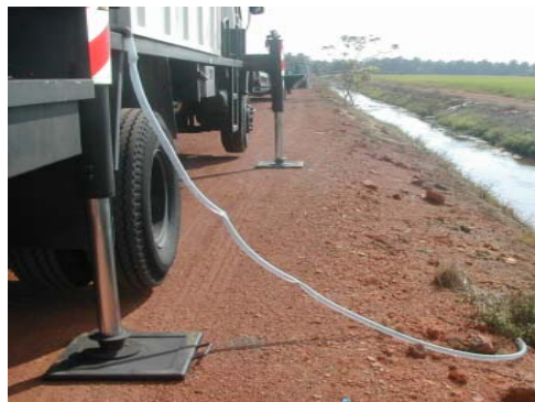
Fig. 1 : Stabilizer as vibration damper.
