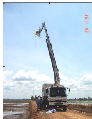
Fig 8: MSS-Mobile Scatterometer System collecting backscattering data in the paddy field.
