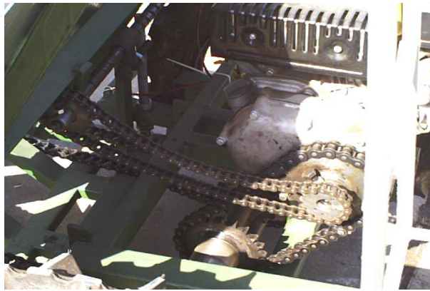
Fig. 10. Photograph of the power transmission system
