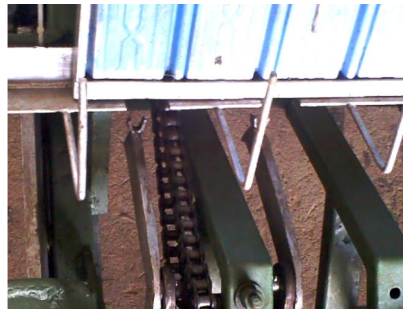
Fig. 8. Photograph of the seedling platform who manufactured to use with seedlings trays.
