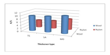
Fig.2. Type of thickener effect on K/S of printed fabrics. (TS: synthetic thickener, SA: sodium alginate, MG: Meypro gum)
