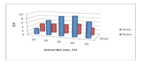
Fig.1. K/S dependence on dye extract concentration.
