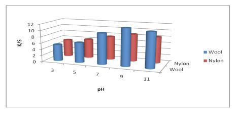
Fig.3. effect of printing recipe pH on printed fabrics K/S.
