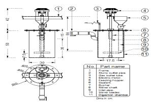
Figure 1a. Elevation, side view and plan of one digester
