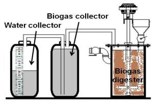
Fig. 2. The biogas measuring method using water displacement system.
