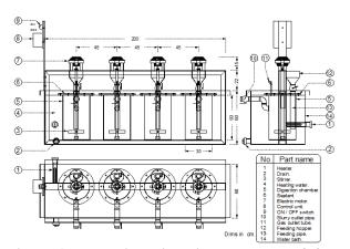
Figure 1b. Elevation, side view and plan of four digesters
