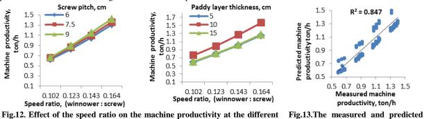
Fig.12. Effect of the speed ratio on the machine productivity at the different screw pitches and paddy layers thicknesses.
