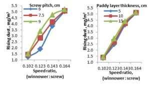
Fig.16. Effect of the speed ratio on the packing rising dust at the different screw pitches and paddy layers thicknesses.
