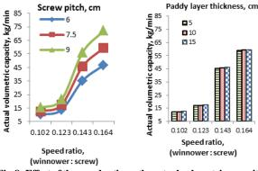
Fig.8. Effect of the speed ratio on the actual volumetric capacity of the conveyor screws at the different screw pitches and paddy layers thicknesses.
