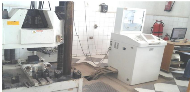
Fig. 5. The universal testing machine with its control unit.
