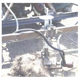
Figure 1. the spiral share with rotary axis
