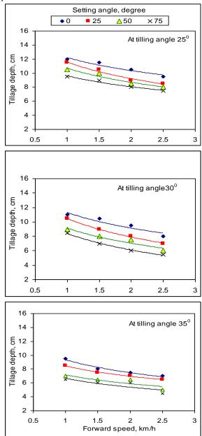
Fig. 9. Forward speed effect on tillage depth.
