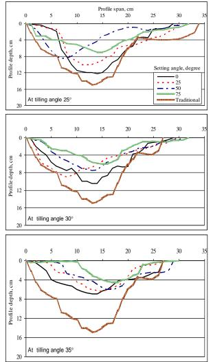
Fig. 8. Tillage profile at different tilling angle.
