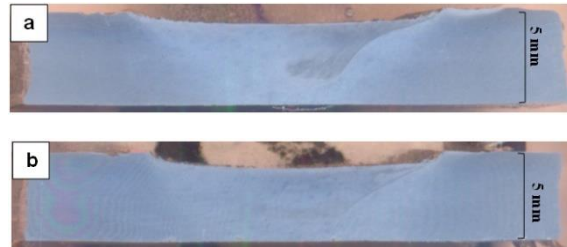
Fig. 3 Optical Macrographs of AA7075/Graphite MMC produced by FSP at 800 rpm after 1 st (a) and 2 nd pass (b)
