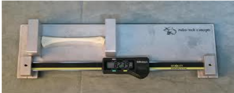
Figure (1): Digital caliper having 0.01 millimeter (mm) sensitivity (Mitutoya).
