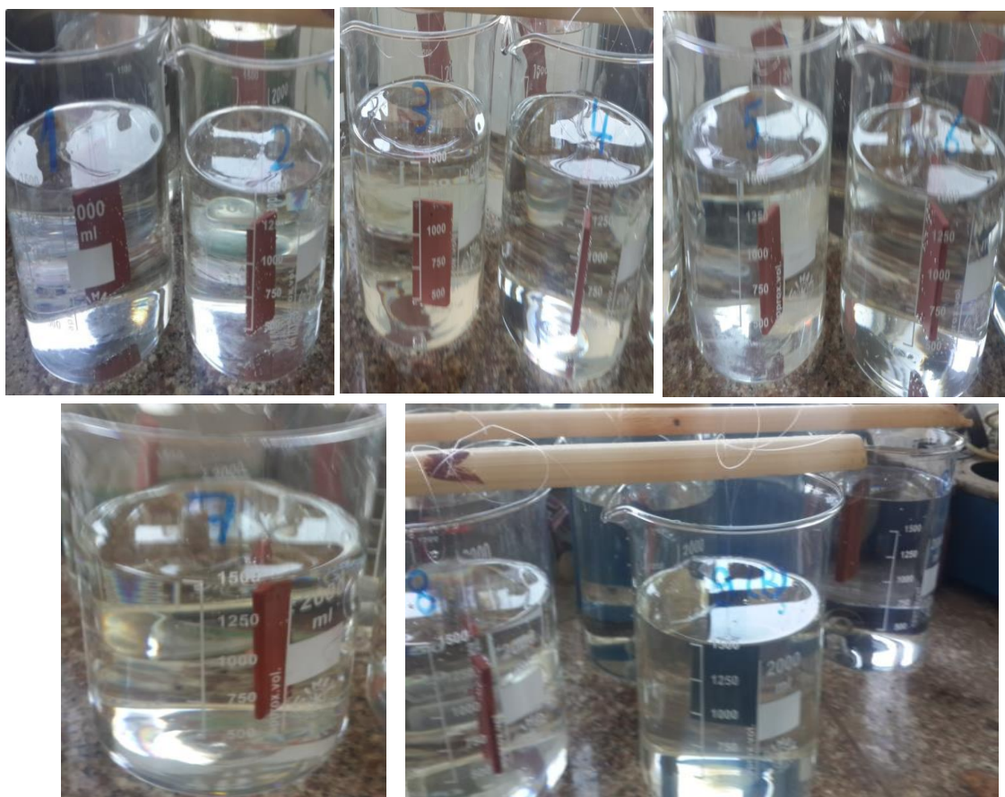
Fig. 1: Zero time wood panels immersed in seawater
