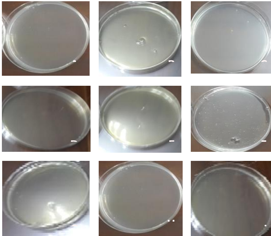
Fig. 3: Bacterial plate count for the slime film on the tested wood panels after four weeks of the immersion in the seawater. A: Corallina mediterranea , B: Codium tomentosum , C: Ulva lactuca , D: Ulva fasciata , E: Pterocladia capillacea , F: Jania rubens , G: Colpomenia sinuosa , H: Artificial paint (R1) and J: Artificial paint (R2)
