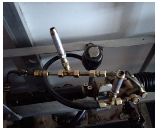
Fig.5 Mounting & adaptation of the used pressure sensors
