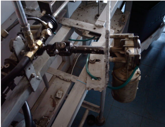
Fig.6 Mounting & adaptation of the used DC motor
