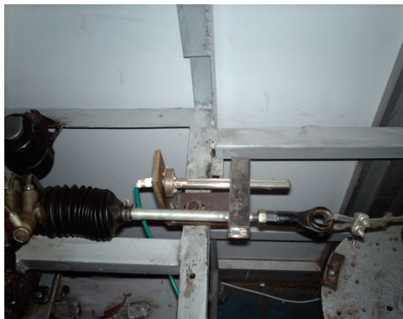
Fig.4 Adaptation of displacement sensor to the rack (Tie rod).
