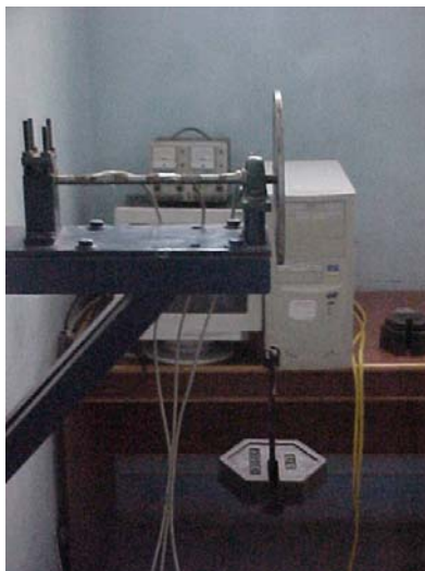
Fig.7. mounting and fixation of (a) fixed support (b) roller support
