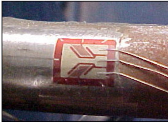
Fig.10. Photography of metal foil strain gauge type KFG-2-120-D31-11 mounted on the measured bar
