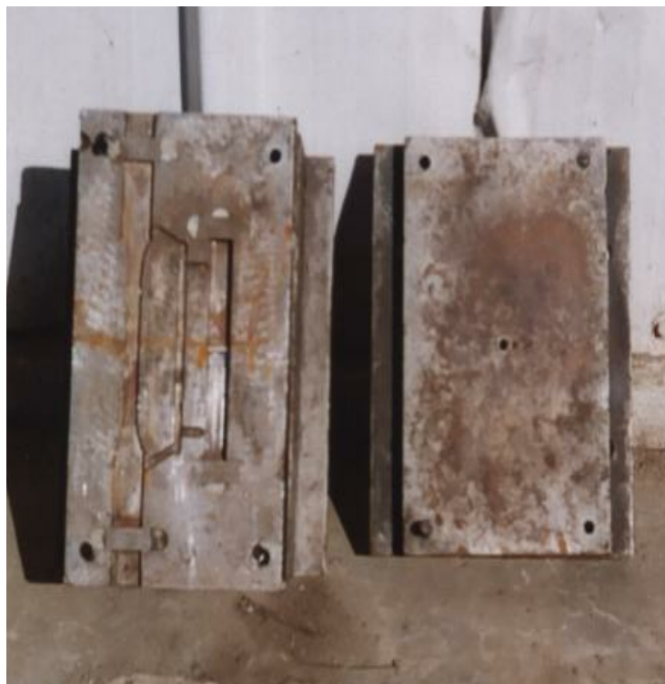
Fig. 2. The manufactured steel die
