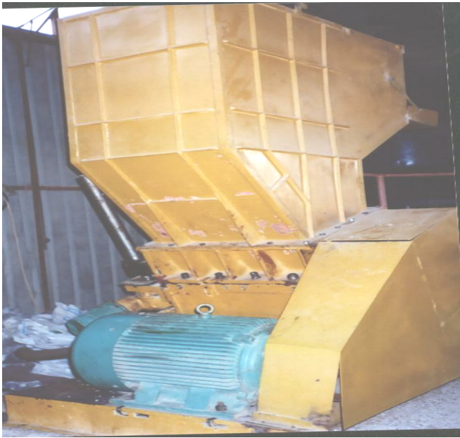
Fig. 4. The plastics crusher
