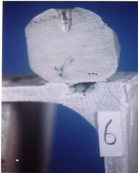
Fig.9 The photography of the large “L” with spherical riser when casting was between the pouring gate and the riser was beside the casting.
