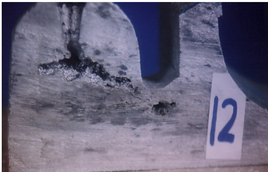
Fig.13 The photography of the small “L” with blind elliptical riser located beside the casting.
