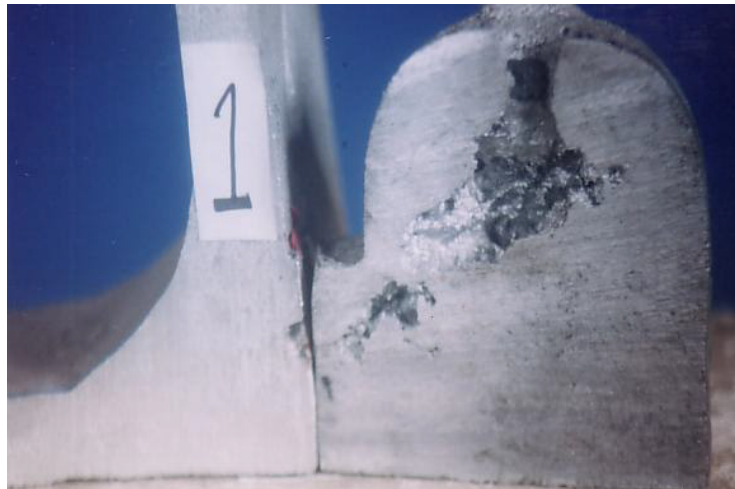
Fig .6 The photography of L (large section) on placing the elliptical riser between the casting and the pouring gate
