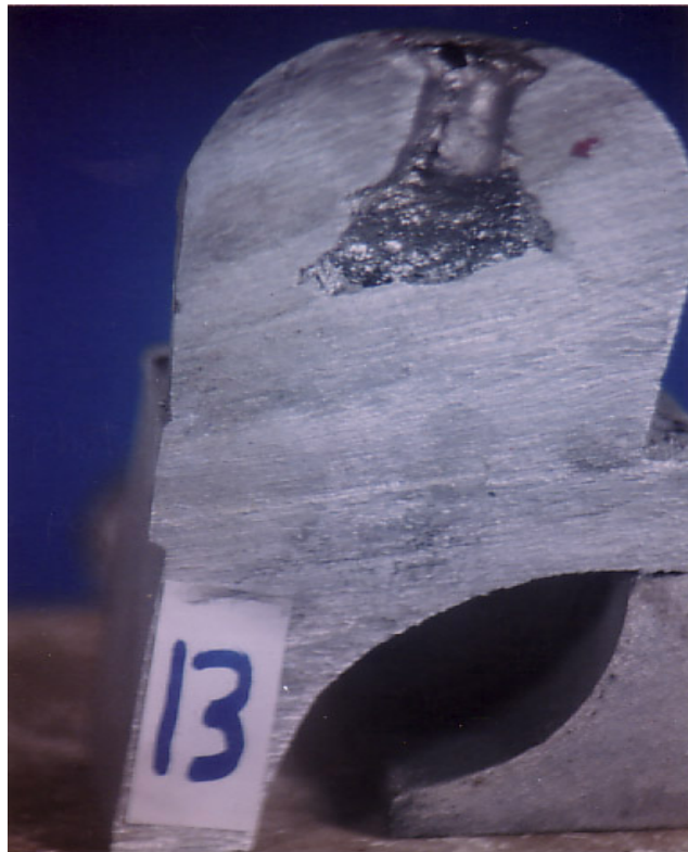
Fig.14 The photography of the small "L" with spherical riser and the riser is between the pouring gate and the casting
