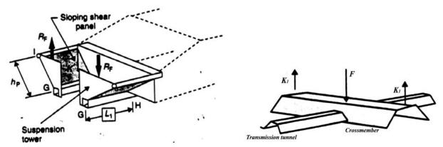
Fig. 9. Sloping the wheel panel assembly Fig. 10. Stiff cross-member and flexible tunnel floor arrangement (load transmitted to sides).
