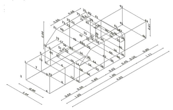
Fig .12. "DOGAN" car body structural model.
