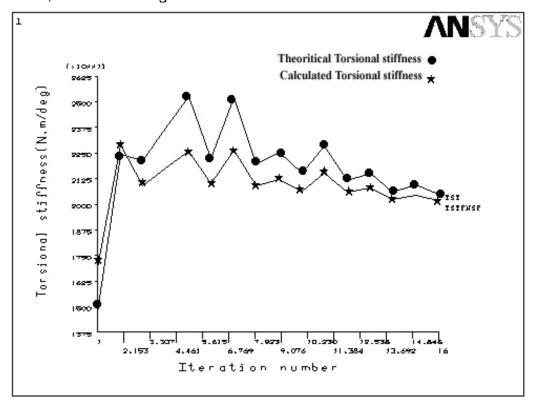
Fig .14. Comparisons between the calculated and theoretical total torsional stiffnesses variation during optimization looping, Torsion Case.
