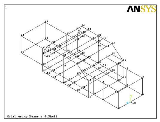
Fig.13. Three-Dimensional model FEM idealization using general shells and beams.
