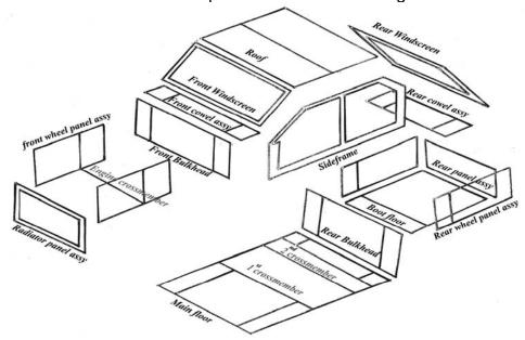
Fig.11. Three-Dimensional representative structural model idealization for a generic
