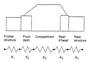
Fig. 8. Structure represented as a series of sub-assemblies.
