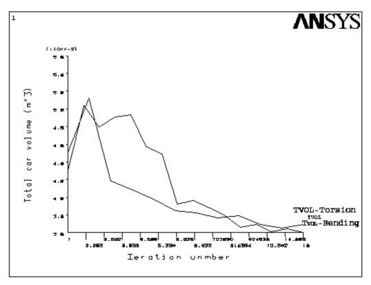
Fig. 15. Comparison between the total car volume variation during optimization looping in both Bending and Torsion cases.
