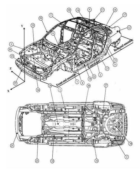
Fig. 1. Body shell assembly for a saloon monocoque closed integral structure.
