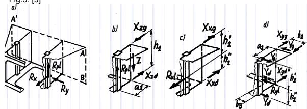
Fig.3. Introduction of forces into the front bulkhead by means of a built up wings; b-vertical; c-longitudinal loads; d-Side loads. Showing the internal shear forces. and the corresponding reactions on the surrounding shear panels.
